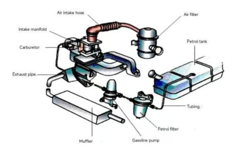
The principle of the gasoline filter is that when gasoline flows through the filter sedimentation cup, the impurities in the gasoline are separated from the water under the action of pressure. The gasoline then passes through the filter material of the filter element to filter out the tiny impurities and water in the gasoline oil, and the gasoline reaches a clean level that can be used by the engine.
